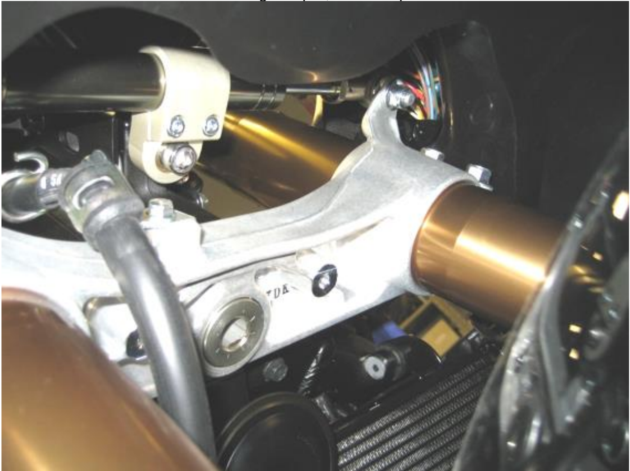
Mounted Steering damper, view w/o plastic cover
